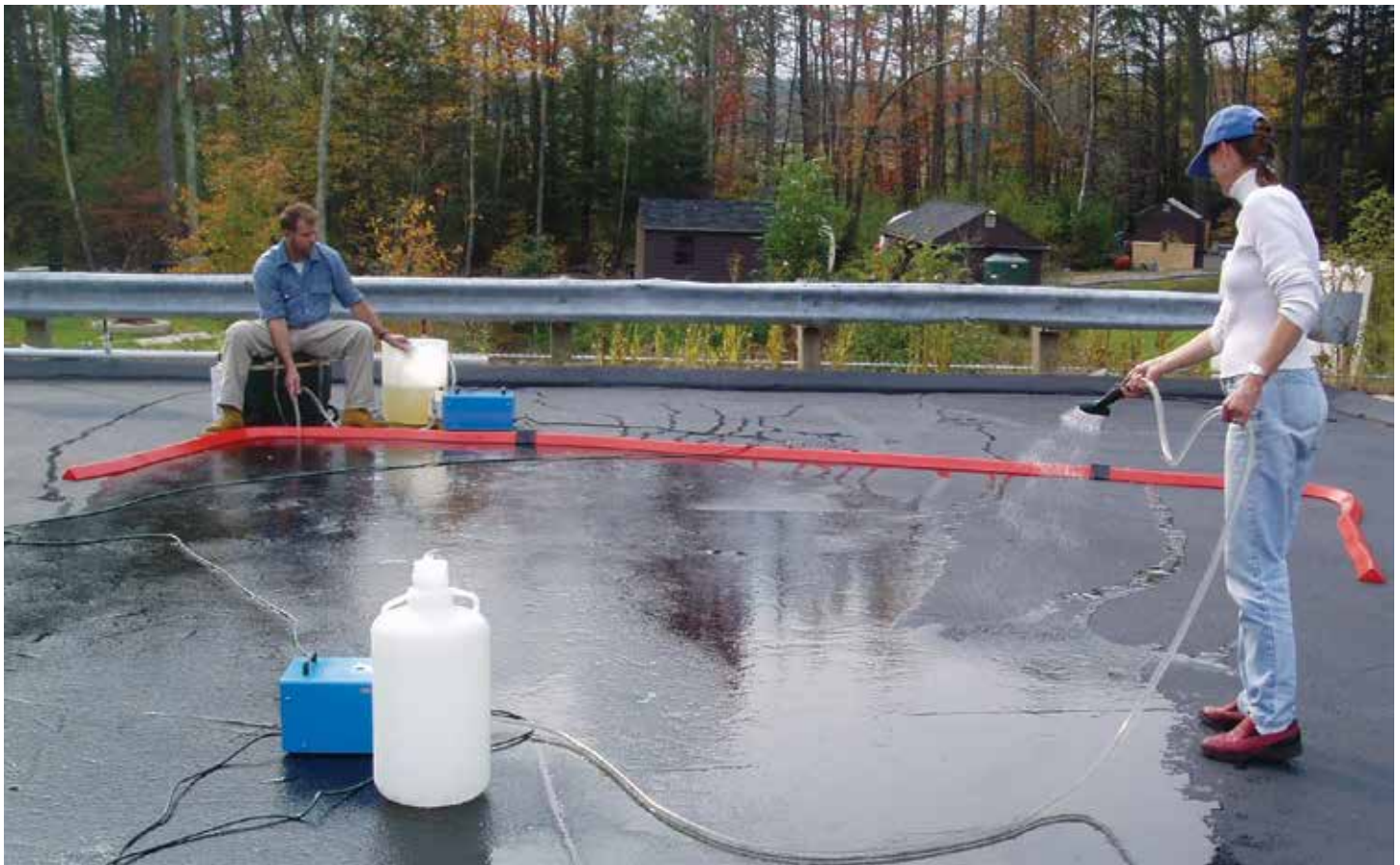
Figure 5. Researchers at the University of New Hampshire Stormwater Center simulate runoff on coal-tar-sealed pavement for measurement of polycyclic aromatic hydrocarbons (PAHs). Photo by the University of New Hampshire Stormwater Center.
