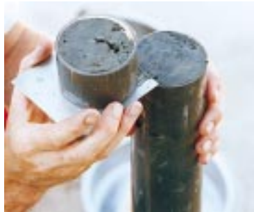
Removal of a 5-centimeter subsample of the sediment core for laboratory analysis.
