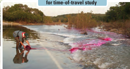
Release of Rhodamine dye for time-of-travel study
