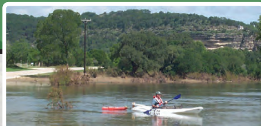
Measuring stream discharge during flood using tethered acoustic Doppler current profiler
