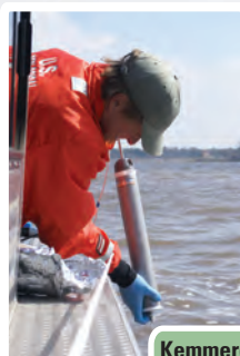
Kemmerer (depth specific) water-quality sampling
