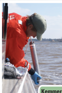
Kemmerer (depth specific) water-quality sampling
